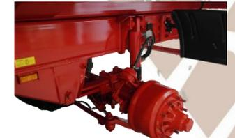
Suspension hydraulique paraboles
